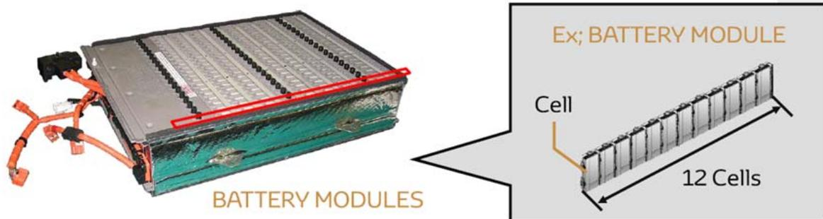
NOTE: DC 201 - 288 V = 1.2 V x X cells x Y modules)
