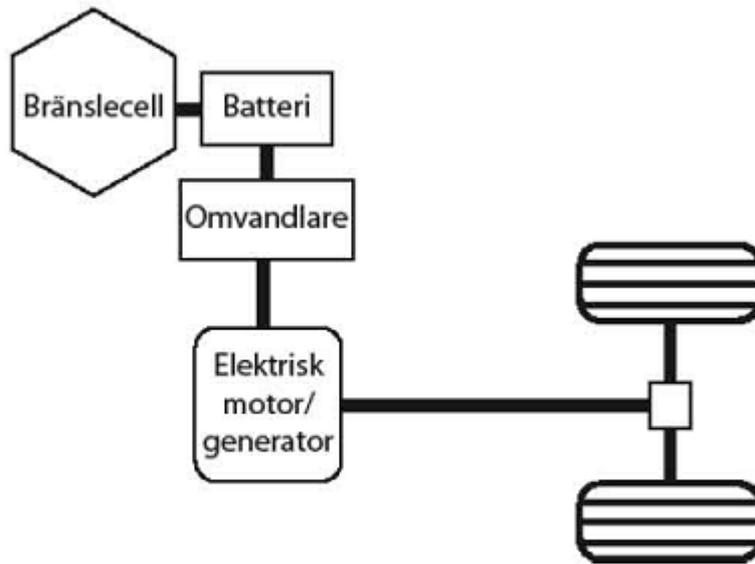
A fuel cell car is driven by fuel cells that generate current for an electric motor. The concept is very similar to a hybrid car, with the difference that it is a fuel cell that generates current instead of a combustion engine.
