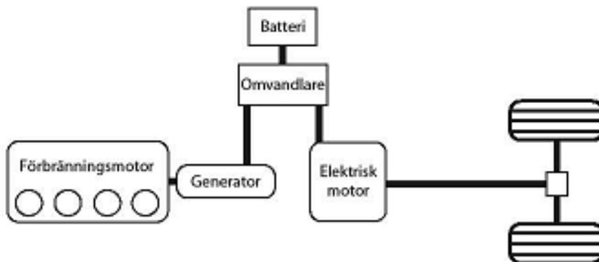
In a series hybrid the combustion engine is connected to an alternator that charges the electric motor's batteries. Then the car is driven by the electric motor. The series hybrid can simply be described as a car that is driven by electric power and that obtains almost all of its electric power from a combustion engine.
