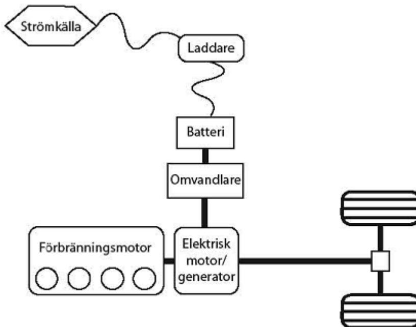
A charge hybrid car is a hybrid car that also can be charged in an electric power outlet – a combination of a hybrid car and a battery car. Thanks to the electric power outlet, the batteries can be charged without the combustion engine, which means that fuel can be saved. However, there is still a combustion engine in the car and it is started when the battery is discharged and when extra power or range is needed.
