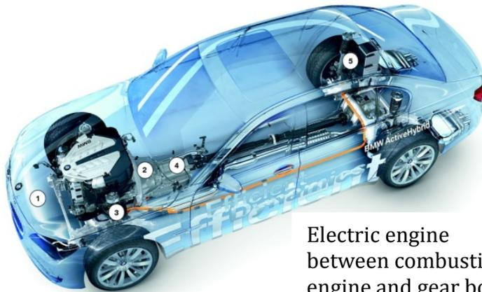
Electric engine between combustion engine and gear box
