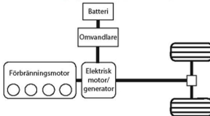
In a parallel hybrid the combustion engine can, by way of the alternator, charge the electric motor's battery and may also be connected to the drive axle via a transmission. This means that the combustion engine can drive the wheels and, when all energy from the combustion engine is not needed for the wheels, the electric motor can work like an alternator and charge the batteries.
